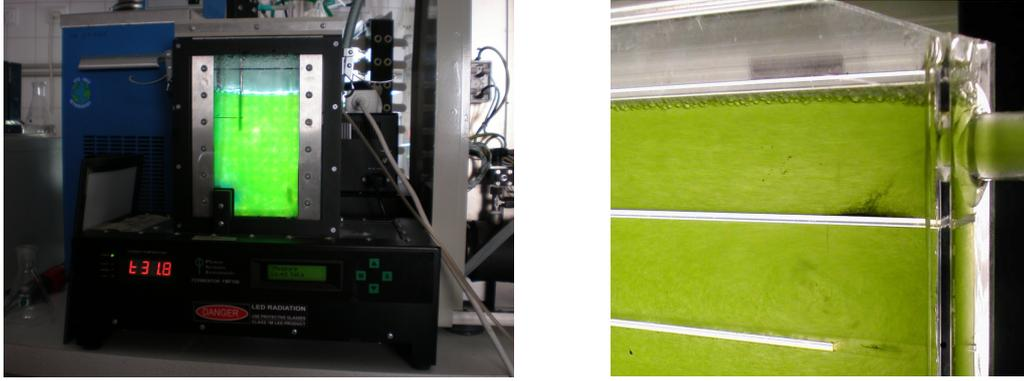
Figure 1: Two examples of rectangular PBR geometry: Photobioreactor FMT 150, made by Photon Systems Instruments, Czech Republic, [www.psi.cz](http://www.psi.cz) (left), and Flat panel photobioreactor, Institute of Physical Biology, University of South Bohemia, Nové Hradý, Czech Republic (right).
