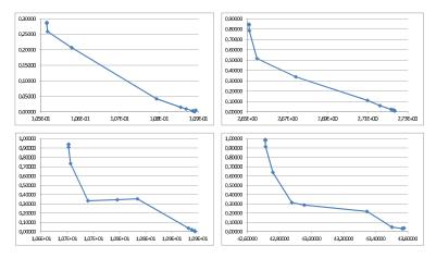
Neumann boundary condition, noise = 1%, 5%, 10%, 20%: L-curve – values J against values  $\omega$  $\alpha$  = 0, 1d-4, 1d-3, 1d-2, 1d-1, 5d-1, 1, 5, 10, 50, 100, 500
