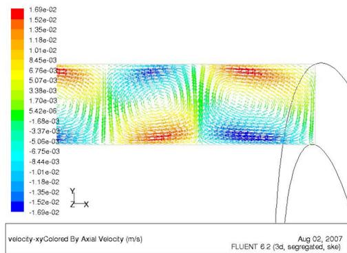
Fig.2: Flow field in axial section of Couette-Taylor PBR computed by CFD code Fluent, Papáček et al. (2007b).
