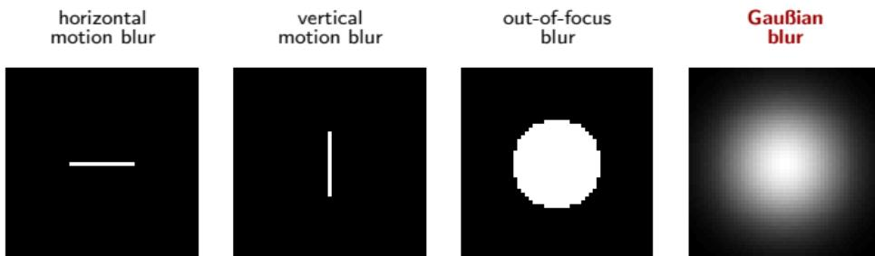
(Note: Action of the linear and spatial invariant blurring operator  $\mathcal{A}(X)$  on the given image  $X$  is done by **2D convolution** of the image with the PSF corresponding to the operator.)
