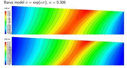
Flow in a converging channel Barus model  $\nu = \exp(\alpha \pi)$ ,  $\alpha = 0.3061$
