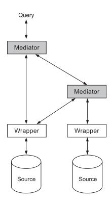
Figure 1: A mediation integration architecture
