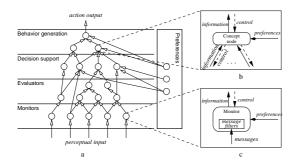
Fig. 1. Architecture —network of concepts (a); Concept node (b); Monitor (c)
