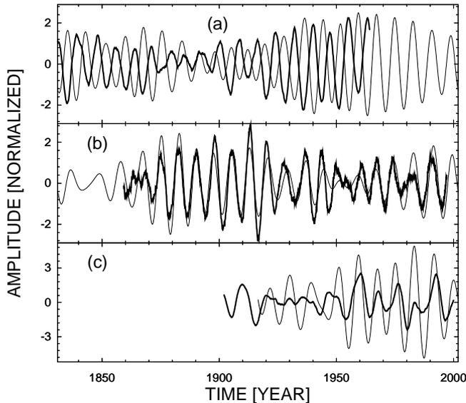
Fig. 3. The oscillatory modes with the mean period 96 months extracted by using SSA (thick lines) and CCWT (thin lines) from the near-surface air temperature (a), the NAO index (b), and the aa index (c).
