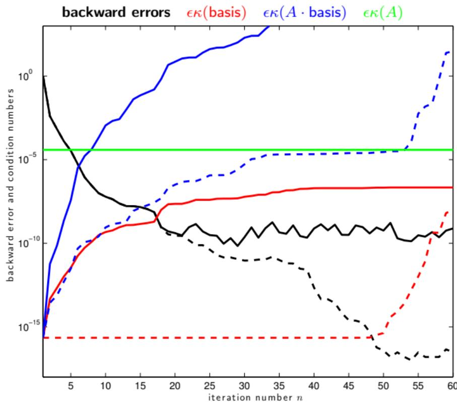
FS1836,  $b = A(1, \dots, 1)^T$ : Simpler GMRES fails, adaptive wins
